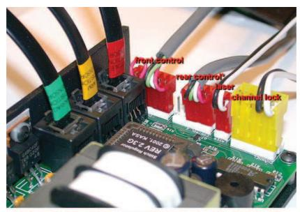
\* the four pin connector should be aligned right, leaving two pins empty on the left
