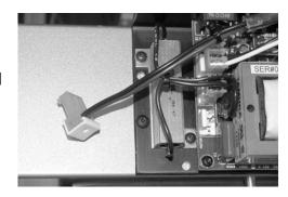
Plug the motor connector in the header of the surge protector module, and insert the module's connector in the motor header, as the picture shows.
