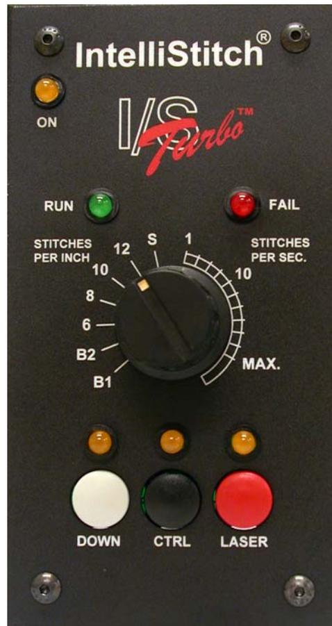
The "FAIL" light serves as a warning light. If it flashes when you are using regulated stitching mode, it is indicating that the stitches have reached twice the chosen length and you are moving the machine too fast. It will be continuously lit when the controller detects a needle jam.
