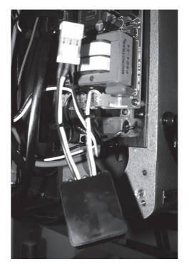
Replace the back cover. Push the surge protector and the motor cable connector into the cover as the picture shows. Arrange the phone cables inside the notches on the bottom and the left side before tightening the bolts.
