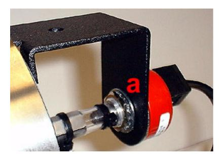
The needle position sensor is placed on the rear shaft of the motor. The sensor is mounted on
