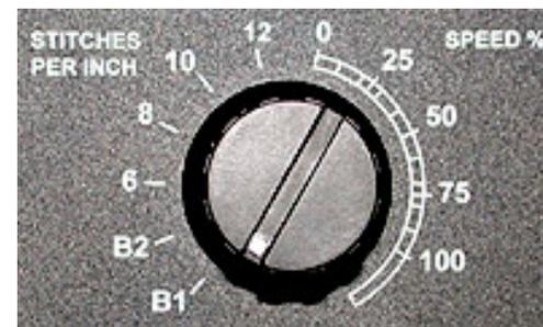
1. Check the speed and strength of the needle movement. The proper setting should provide just enough strength to stitch through the fabric going down and pull out going up without jamming. Avoid setting the needle speed too high, for it may cause the needle to run over its top and bottom position.
